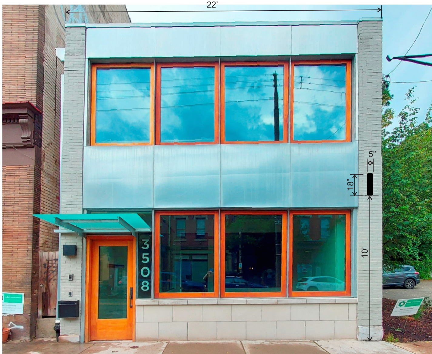
FRONT ELEVATION - Sign Type (1)(QTY:1) D/F Projecting Sign - Flag Mount Scale: 1/4" = 1' (5.2 SQFT)
