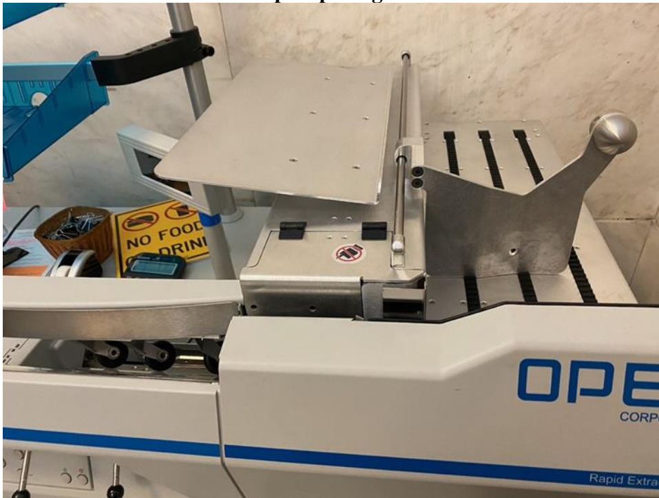
PHOTO 4 CITY REAL ESTATE TAX BILL PROCESSOR OPEX FalconV+ Envelope Opening Section
