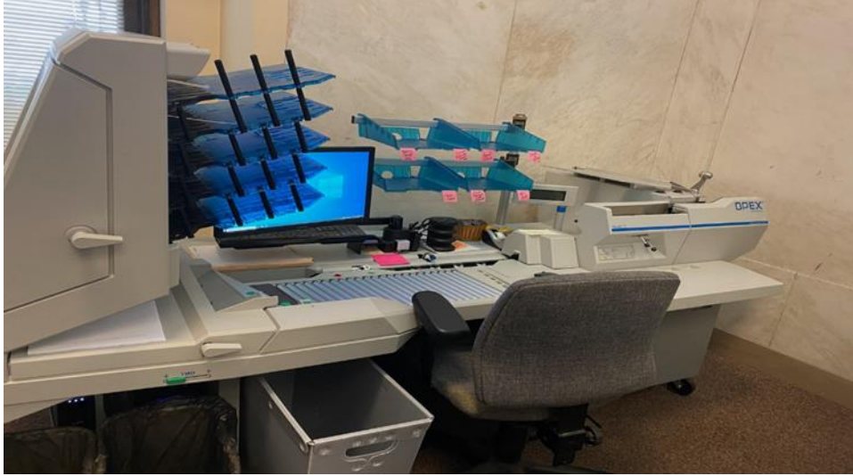
PHOTO 3 CITY REAL ESTATE TAX BILL PROCESSOR OPEX FalconV+ Envelope Opening, Image Scanning, and Storage
