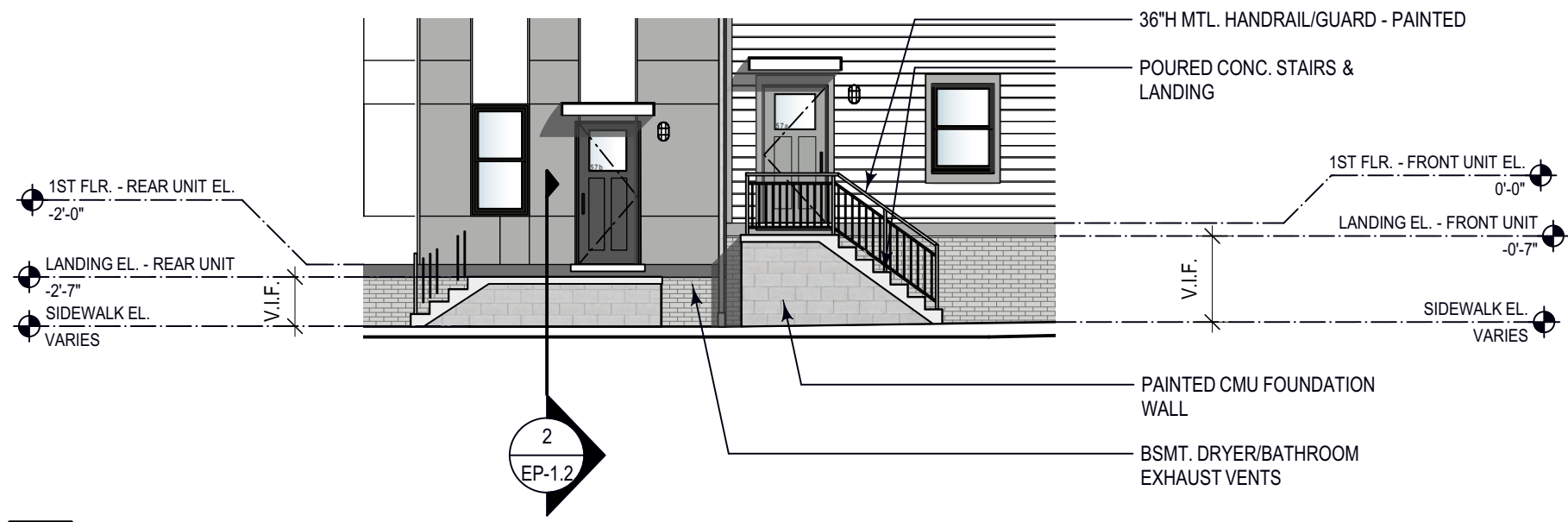
1 PARTIAL ELEVATION - UNIT ENTRY LANDINGS Scale: 1/8" = 1'-0"
