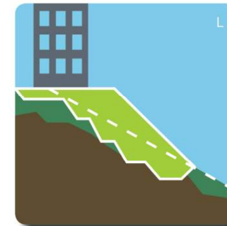
Extending Fill Embankments
