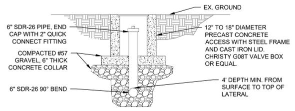
**DRAIN CONNECT & PRECAST CONCRETE ACCESS**
